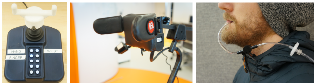
Figure 1: Control interfaces used in this study. From left to right : 3-axis joystick, head array system, sip/puff switch.
