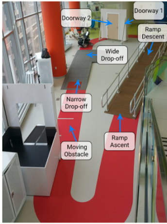
Fig. 3: Wheelchair navigation track. Tasks include doorway traversal, ramp descent and ascent, drop-off avoidance, and dynamic obstacle avoidance.
