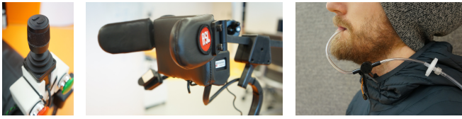
Fig. 1: Control interfaces used in this study. From left to right: 3-axis joystick, head array system, sip/puff switch.
